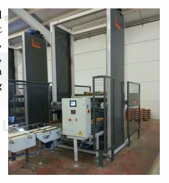
The PLC has inputs and outputs for automatic connection to manual packing tables or place packer machines.
