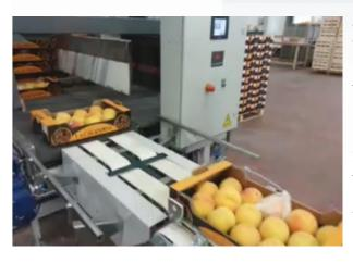
Rotator at the table entrance: If you have a barcode traceability system, the palletizer can rotate the boxes so the barcode is always at the visible side of the pallet.
